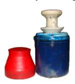
You can grease pack bearings two different ways. One, place a large dollop of grease on the palm of your hand with your other hand push the bearing into the grease until you see grease coming out of the other side of the bearing. Two, using a "bearing packer" place bearing on the piston press down on cap until grease shows on top of the bearing. This is more effective with less mess.
